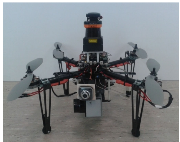
Fig. 3 NUS quadrotor platform with two onboard laser range finders
